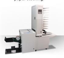
EC-4800 can be connected to most of the mainstream booklet makers in the market to easily produce booklets as an on-line finishing process. By connecting the twin-tower (EC-4800/EC-4800L) to a booklet maker, it is able to produce a maximum of 80 pages booklet.
