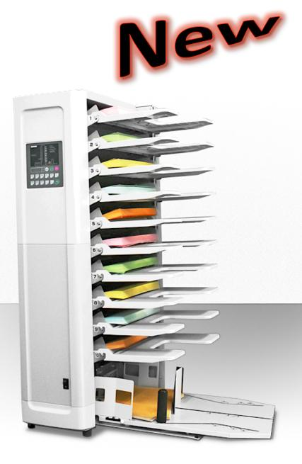
The most capable desk-top collator features the highest speed among the 10-bin table-top collators processing 4,200 sets per hour for A4 size papers. The machine al-so detects paper jams, miss-feed, paper level in the receiving tray, empty bin condition and paper thickness in order to prevent double feeding, and automatically stops while displaying the nature of the faults. EC-4800 is able to handle a wide range of papers from post-card to SRA3 size papers.
